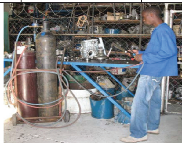
Easy: slicing through steel with an oxy-acetylene flame.
