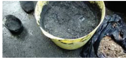
Fig.10 Mixing Charcoal dust, soil & water
