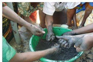
Fig. 13. Molding the mixture into briquettes
