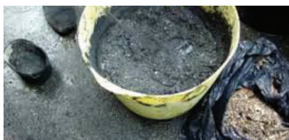
Fig. 10. Mixing Charcoal dust, soil & water
