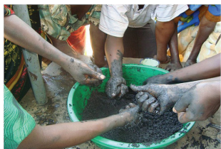
Fig. 13. Molding the mixture into briquettes
